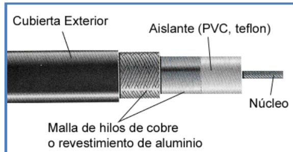
**Figura 2.9:** Partes cable coaxial
