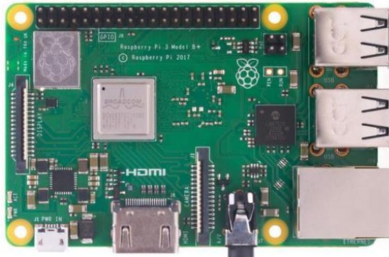
FIGURE 20 IMAGEN DE RASPBERRY PI 3 (RASPBERRY, 2022)
