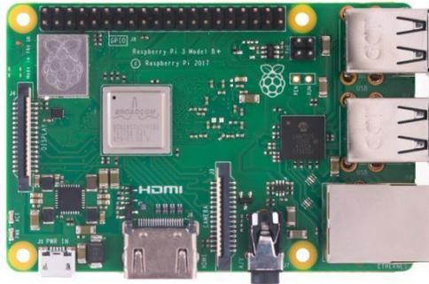
Figure 32 RASPBERRY PI 3 MODELO B+ (RASPBERRY, 2022)
