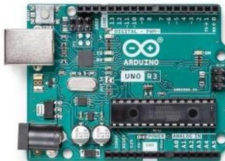
FIGURE 11 IMAGEN DE ARDUINO UNO R3 (ARDUINO, Arduinon UNO R3 , 2023)
