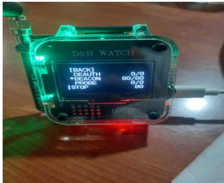
Figura 40: Ataque “Beacon Flooding”
