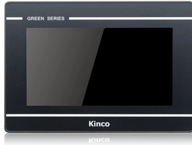
Figura 19: HMI Kinco GL070E [26].
