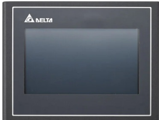
Figura 13: Pantalla HMI DELTA DOP-103BQ [16].
