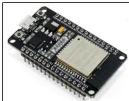
*Figura 11. NodeMCU-32 [39]*
