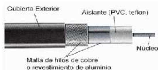
Figura 2.12. Cable Coaxial
