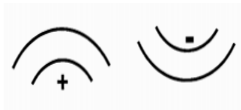
Figura 3.12: Formas de dogleg. Fuente: (Mitchell , 1995) Advance Oilwell Drilling Engineering.
